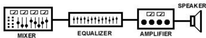
FIG. 11 Monitor Bus that Feeds Only One Monitor Speaker
