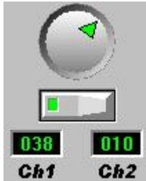
The only practical way to eliminate an input “clip” condition is to reduce the gain of the TEF25. The input gain setting is normally controlled by a panel that is accessed through the main menu “Input, Settings” but this is not always convenient. Also, opening this control panel will also stop any existing signal that is currently being generated by the TEF25. We have provided this onscreen control to allow you to quickly correct an input gain problem and remove a hardware clip condition.
